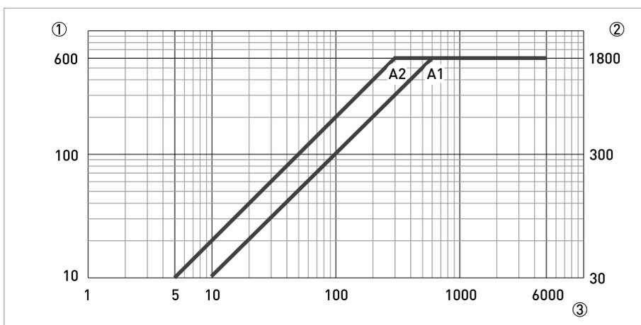
Figure 4-3: Maximum length of signal cable A
