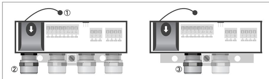
Figure 4-5: Terminal compartment for power supply
