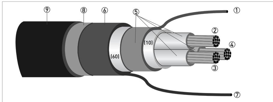
Figure 4-2: Construction of signal cable A (armoured version)
