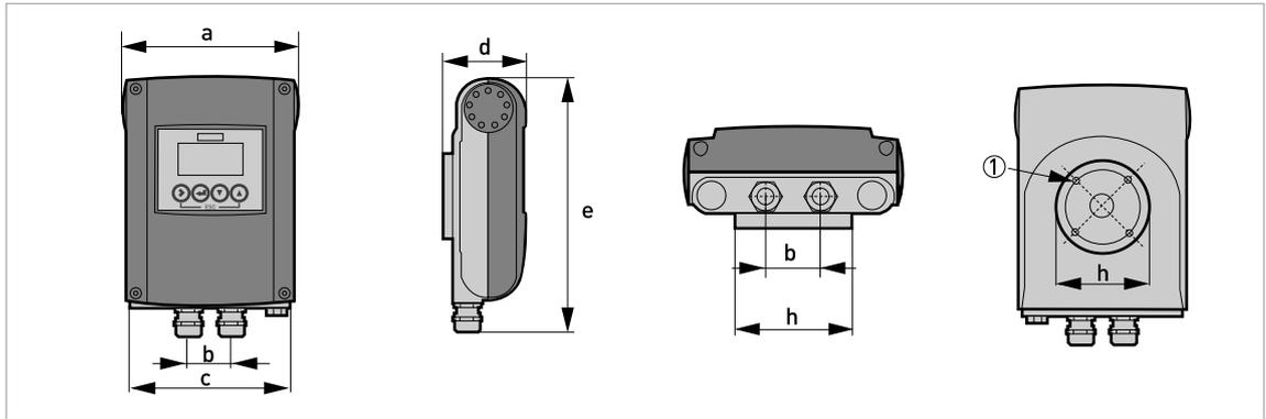
Figure 2-3: Dimensions of compact 0° version, aluminium housing
