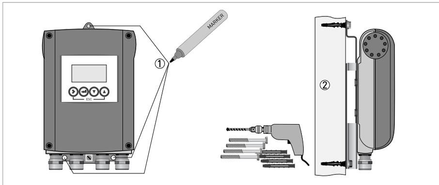
Figure 3-1: Mounting the wall-mounted housing
