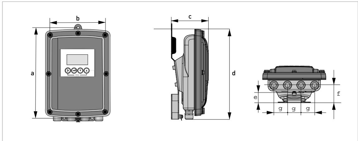
Figure 2-2: Dimensions of wall-mounted and compact 10° version, stainless steel housing
