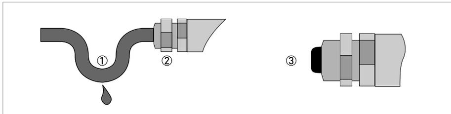
Figure 4-8: Protect housing from dust and water
