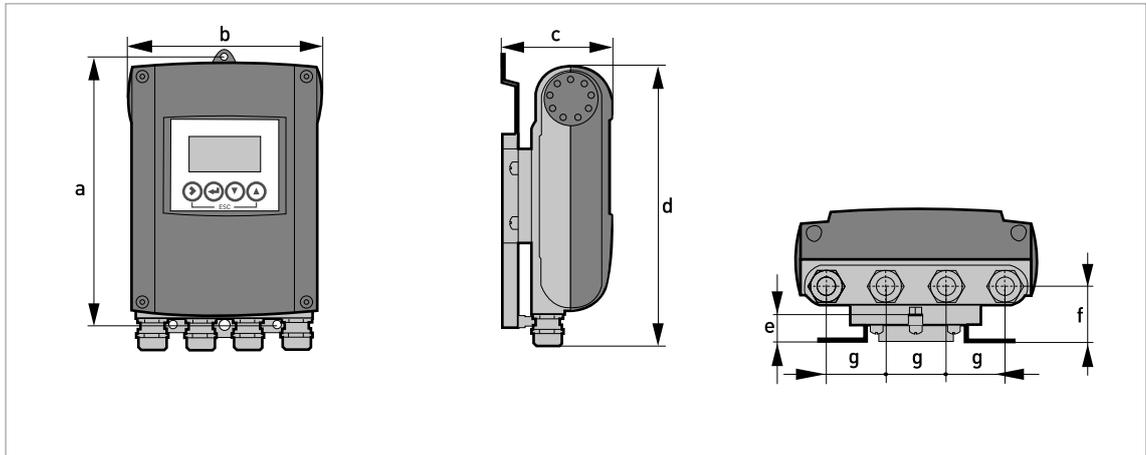
Figure 2-1: Dimensions of the wall-mounted version, aluminium housing
