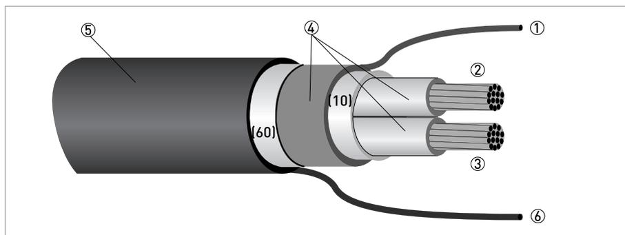
**Figure 4-1: Construction of signal cable A (standard version)**
