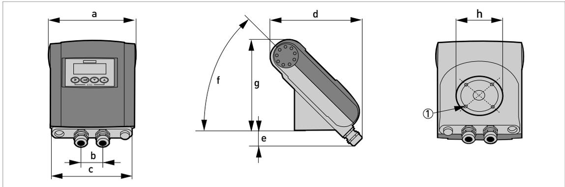
Figure 2-4: Dimensions of compact 45° version, aluminium housing
