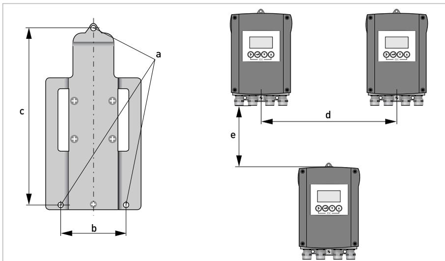
Figure 3-2: Wall mounting of multiple devices (aluminium housing)
