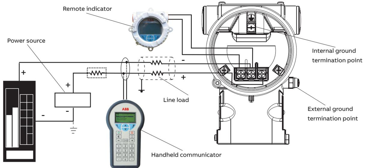
Figure 5 Electrical connection – HART Version
