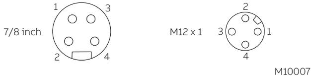
Figure 6 Plug connectors – fieldbus versions
