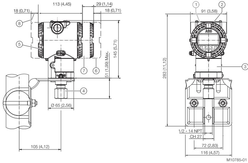
**Figure 2** Dimensions - Barrel housing – 1/2 NPT female thread
