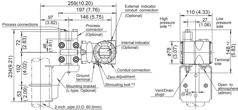
Process connector downside (INSTALLATION CODE '7')
