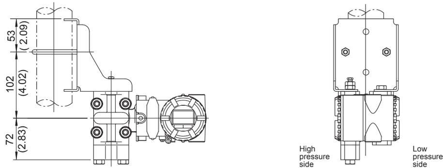
Horizontal Impulse Piping Type (INSTALLATION CODE '9') (For CODE '8', refer to the notes below.)
