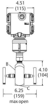
A. Bleed screw (unspecified dimension) - not C. 1/2-14 NPT female NPT process connection (code BA) designed for accessory attachments.
