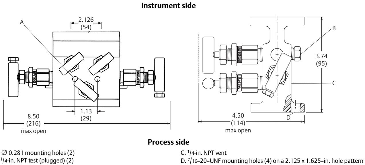
Figure 27. Rosemount 304RW Three-Valve Wafer Manifold<sup>(1)</sup>
