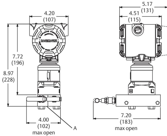
A. 1/2–14 NPT on manifold for process connection, 1/4–18 NPT for test/vent connection
