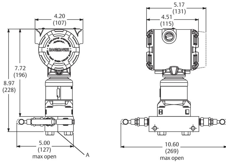
A. 1/2-14 NPT on manifold for process connections, 2 1/8-in. center-to-center, 1/4-18 NPT for test/vent connection
