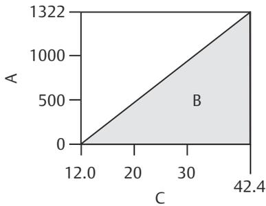
Maximum Loop Resistance =  $43.5 \times (\text{Power Supply Voltage} - 12.0)$
