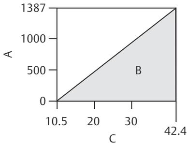
Maximum Loop Resistance =  $43.5 \times (\text{Power Supply Voltage} - 10.5)$
