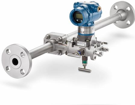
Rosemount 3051CFP Integral Orifice Flow Meters enable highly accurate flow measurement in small line sizes. Internal pipe diameter variation in combination with plate centering issues can greatly magnify flow measurement errors in small line sizes. Integral Orifice Flow Meters use a precision honed pipe section to minimize internal pipe diameter variation along with a self-centering plate design to eliminate alignment errors.
