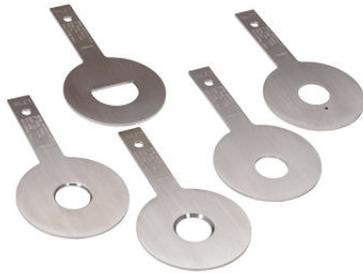
Standard configuration is with a square-edged concentric bore in both paddle and universal type plates. Also available with a machined gasket sealing surface. Final inspection reports illustrating plate thickness, concentricity, outside dimensions, inside dimensions, roundness, and flatness are available.
