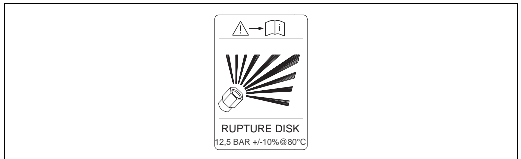
Indication label for the rupture disk
