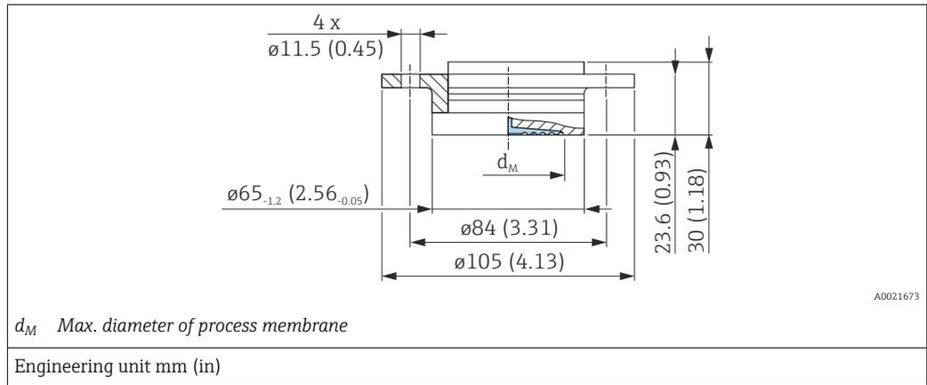
$d_M$  Max. diameter of process membrane
