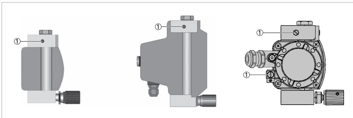
Figure 4-10: Grounding connections
