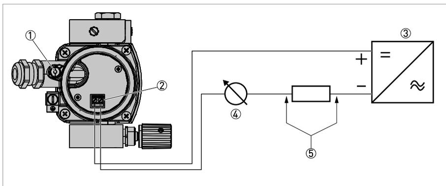
Figure 4-7: Electrical connection of ESK3x
