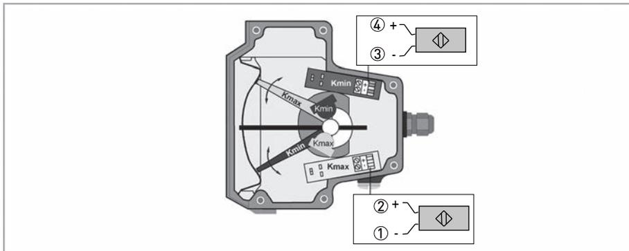
Figure 4-4: Electrical connection of NAMUR limit switches K1/K2
