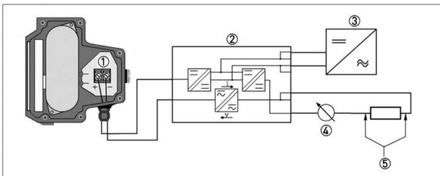
Figure 4-9: Electrical connection with galvanic isolation
