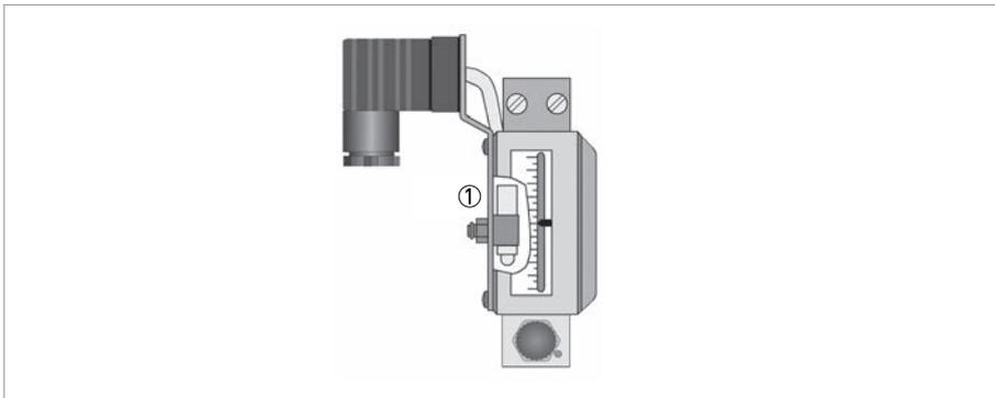
Figure 4-6: Settings of REED limit switch
