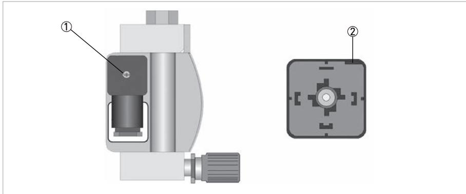
Figure 4-1: Electrical connection of NAMUR limit switches
