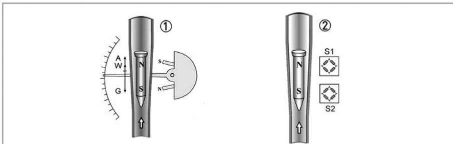
Figure 1-1: Functional principle
