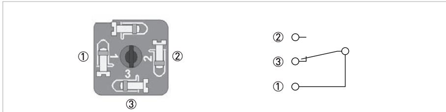
Figure 4-3: Electrical connection of REED limit switch R1
