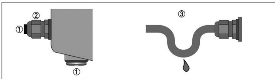
Figure 4-11: Cable feedthrough
