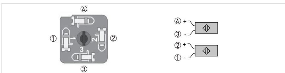
Figure 4-2: Electrical connection of NAMUR limit switches K1/K2
