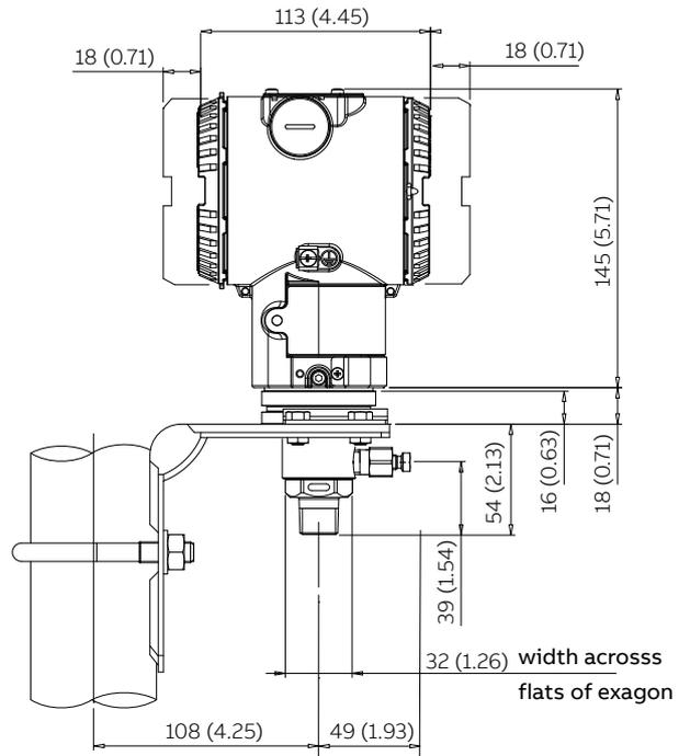
266HSH Transmitter with barrel housing - 1/2 NPT male connection for sensor W
