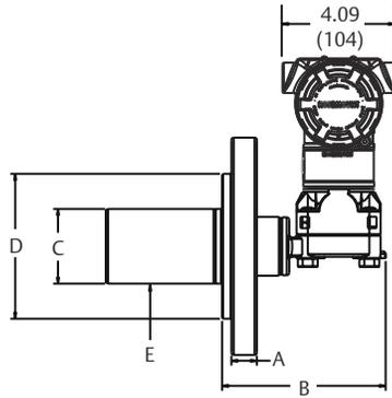
Diaphragm assembly and mounting flange
