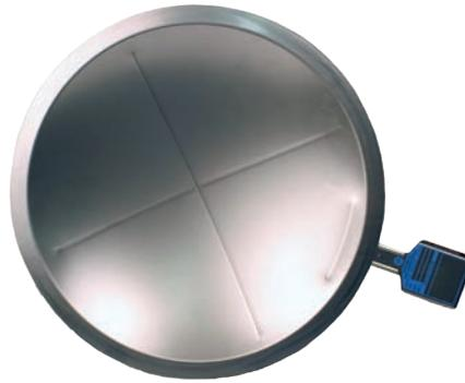
The **RCS Rupture Disc** is a reverse acting, cross-scored, solid metal rupture disc, providing reliable pressure relief protection, and easy installation. It is a non-reclosing differential pressure relief device that provides instantaneous full opening for protection of equipment, vessels and systems from overpressure conditions.
