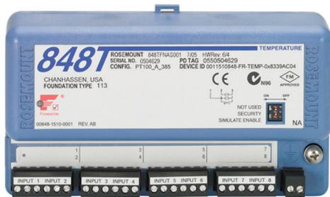
The Rosemount 848T offers a low-cost solution for high density measurements. The transmitter accepts eight independently configurable sensor inputs, and can be mounted close to the process to improve data quality. FOUNDATION Fieldbus architecture allows up to 128 temperature measurements to be transmitted on a single H1 Fieldbus line.
