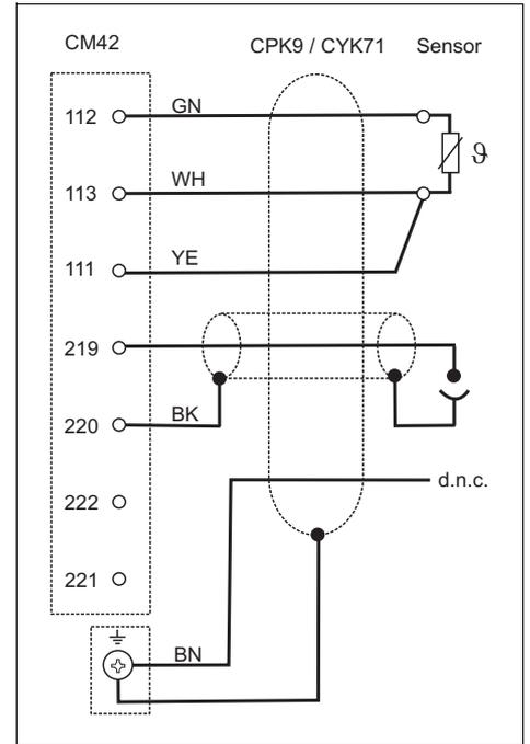
**Conductive sensors, four-electrode sensors**
