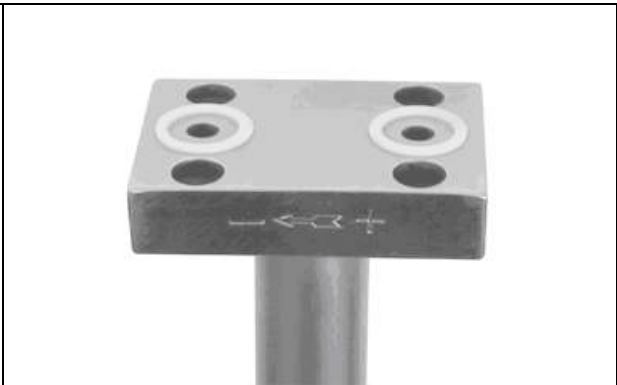
Fig. 34: Sensor head with flange plate to direct-mount a 3-way manifold. Limited use w/out pipe insulation, gases to pressure max = 63 bar (926 psig) and temp max = 200 °C (680°F) liquids to pressure max = 63 bar (926 psig) and temp max = 150°C (510°F)
