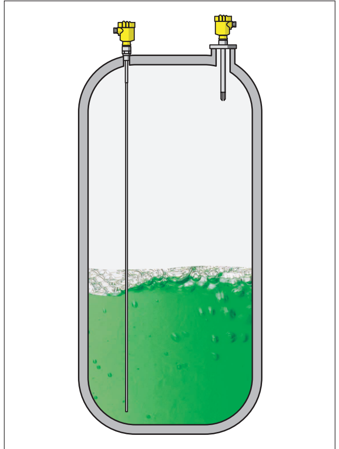
Fig. 2: Level detection in vessels with solvents
