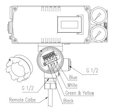
Fig. 5-5: YT-3302 Positioner main body and cables
