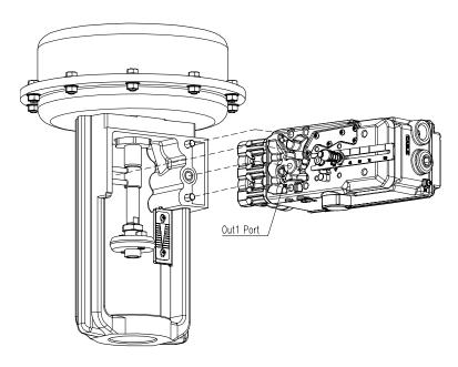
Fig. 3-21: YT-3300 / 3350L(Adapter Lever Type)
