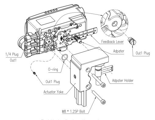
Fig. 3-20: Installing the positioner on the actuator
