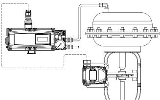
Fig. 4-3: Single acting linear actuator (YT-3301L)
