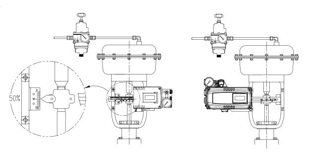
Fig. 3-9: YT-3300L / 3350L (Standard Lever Type)
