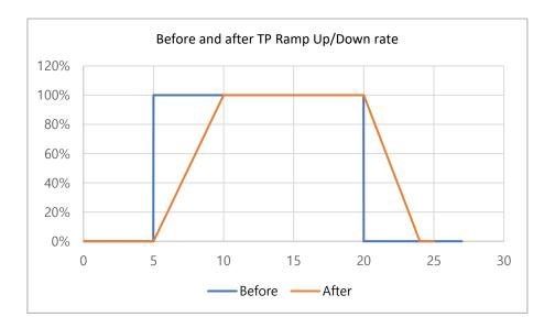
The curves below show the target position (red) and the actual position (blue) of the valve after applying SP Ramp Up/Down rate.
