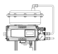
Fig. 4-1: Single acting linear actuator (YT-3300L / 3350L / 3303L)
