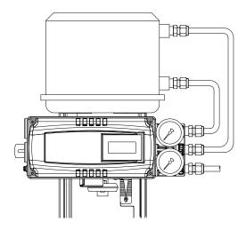
Fig. 4-7: Double acting linear actuator (YT-3300L / 3350L / 3303L)
