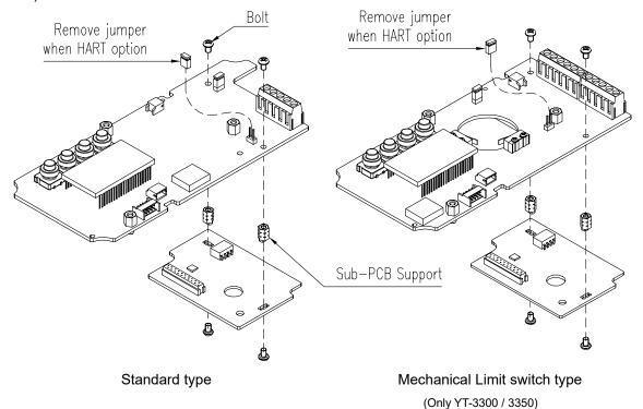
Fig. 7-2: Installation of Option PCB on Main PCBs
