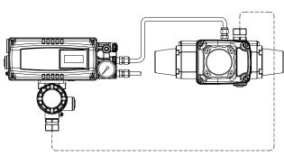
Fig. 4-6: Single acting rotary actuator (YT-3302R)
