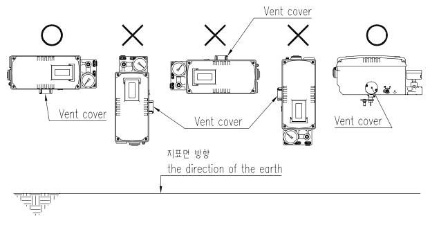
Fig. 3-1: The correct positions of a vent cover
