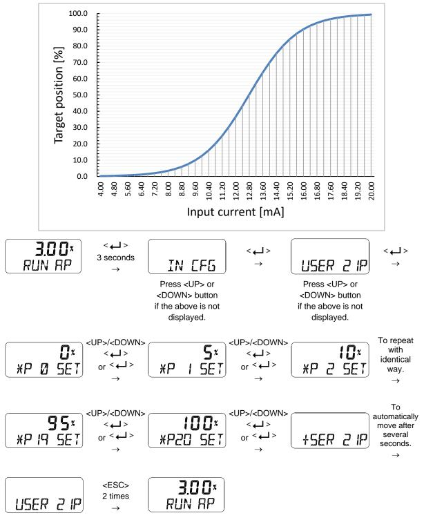
This function is activated by saving the Valve Flow Characterization Curves (CHAR) of above Section 9.9.5 as "U21".
