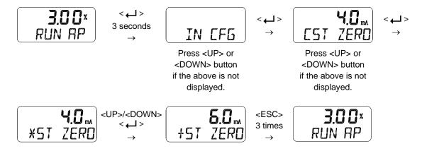
This function is activated by saving the Split Range Mode (SPLIT) of above Section 9.9.2 as "CSt".
