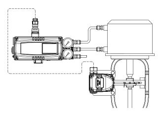
Fig. 4-9: Double acting linear actuator (YT-3301L)
