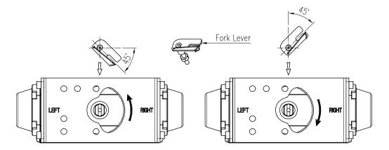
Fig. 3-30: Counter-clockwise and clockwise rotation.
