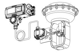
Fig. 3-5: YT-3302L installation example
