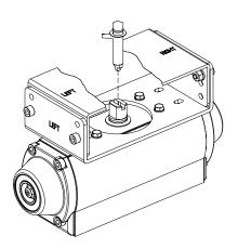
Fig. 3-33: Main shaft center alignment (Namur)
