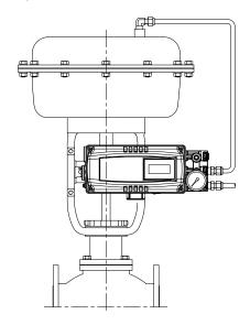
Fig. 3-2: YT-3300L / 3350L installation of standard lever type example
