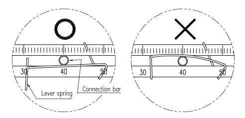
Fig. 3-11: Proper way to insert connection bar between feedback lever and lever spring
