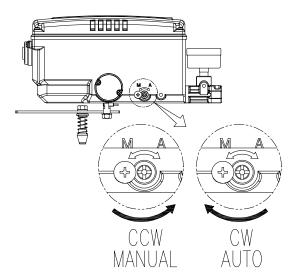
Fig. 6-3: A/M switch adjustment
