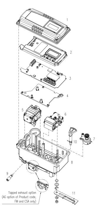
Fig. 2-2: YT-3303 exploded view
