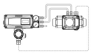
Fig. 4-12: Double acting rotary actuator (YT-3302R)
