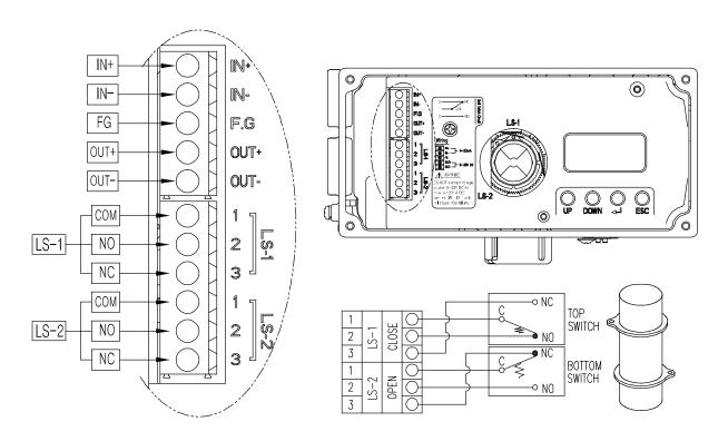
Fig. 5-2: Terminal of two Mechanical Switches (Only YT-3300 / 3350)
