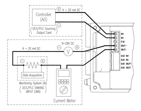
Fig. 9-3: Setting 4-20 mA Analog Output
