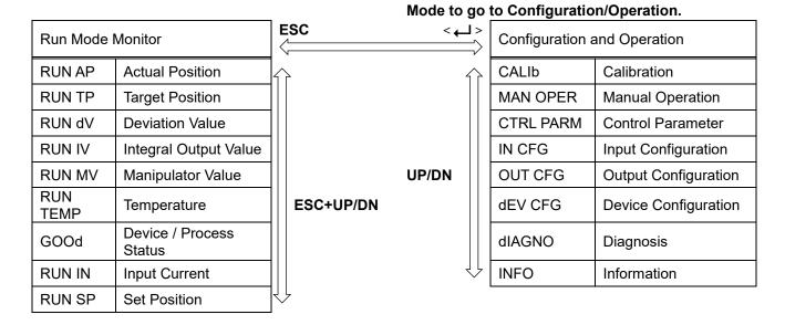
Press the < > button to select the lower menu of the Configuration/Operation menu. Press the ESC button to return to parent menu after completing configuration. Pressing the ESC button anywhere in the menu structure several times returns the user to the uppermost menu, Run Mode Monitor menu.
