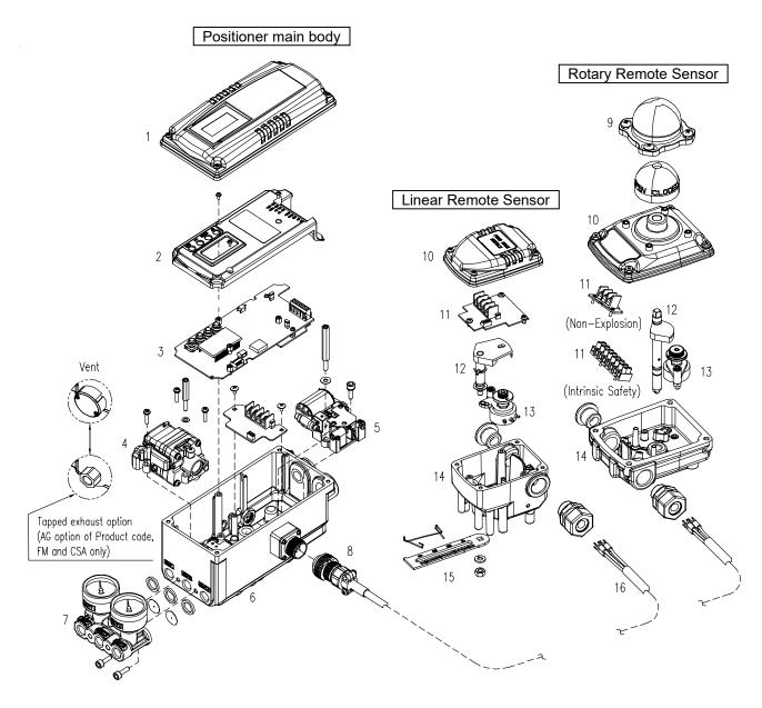
Fig. 2-3: YT-3301 exploded view
