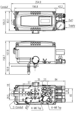
Fig. 2-6: YT-3300L (Adapter Lever Type)
