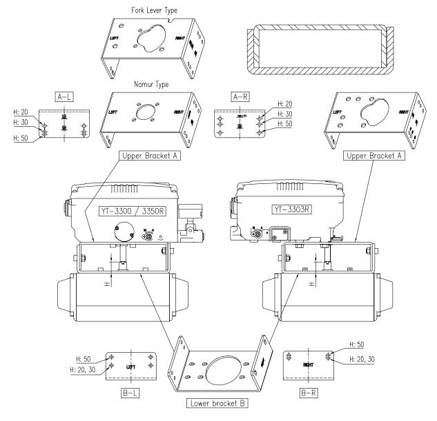
Fig. 3-27: YT-3300R / 3350R / 3303R Brackets and positioner
