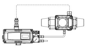
Fig. 4-4: Single acting rotary actuator (YT-3301R)
