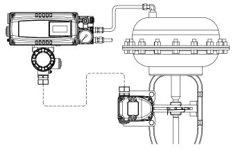
Fig. 4-5: Single acting linear actuator (YT-3302L)
