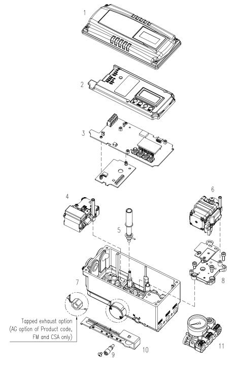
Fig. 2-1: YT-3300 / 3350 exploded view
