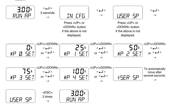
This function is activated by saving the Valve Flow Characterization Curves (CHAR) of above Section 9.9.5 as "U5".
