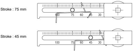
Fig. 3-14: YT-3300L / 3350L Feedback lever and location of the connection bar
