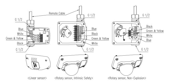
Fig. 5-4: Remote sensor and cables
