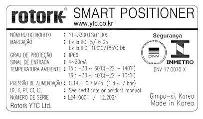
Fig. L-5: YT-3300 / 3303 / 3301 / 3302 Intrinsic safety type (INMETRO)
