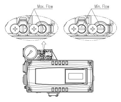
Fig. 6-5: Variable orifice adjustment
