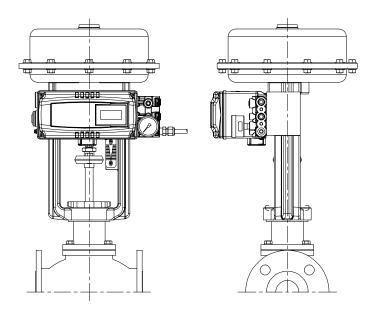
Fig. 3-18: YT-3300L / 3350L installation of adapter lever type example
