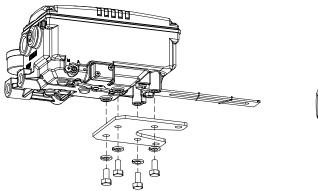
Fig. 3-7: Attaching positioner to bracket (YT-3303L / 3301L / 3302L)
