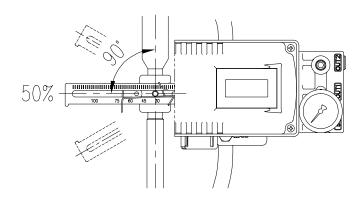
Fig. 3-12: YT-3300L / 3350L Feedback lever and valve stem
