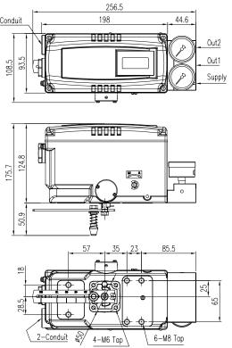
Fig. 2-10: YT-3350L (Adapter Lever Type)
