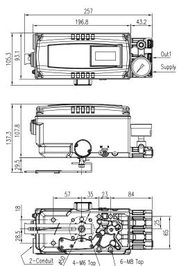
Fig. 2-5: YT-3300L (Standard Lever Type)
