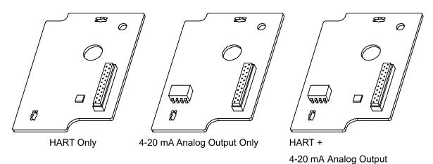
Fig. 7-1: Three types of Sub-PCB
