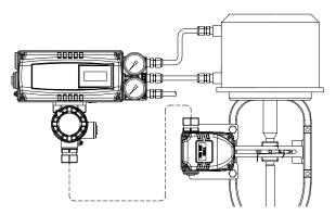
Fig. 4-11: Double acting linear actuator (YT-3301L)
