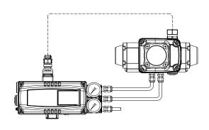
Fig. 4-10: Double acting rotary actuator (YT-3301R)
