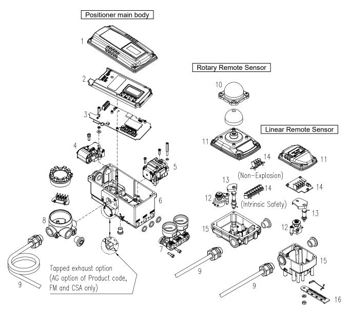
Fig. 2-4: YT-3302 exploded view
