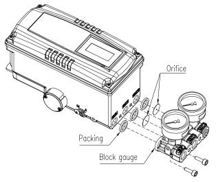
Fig. 6-4: Plate type Orifice installment
