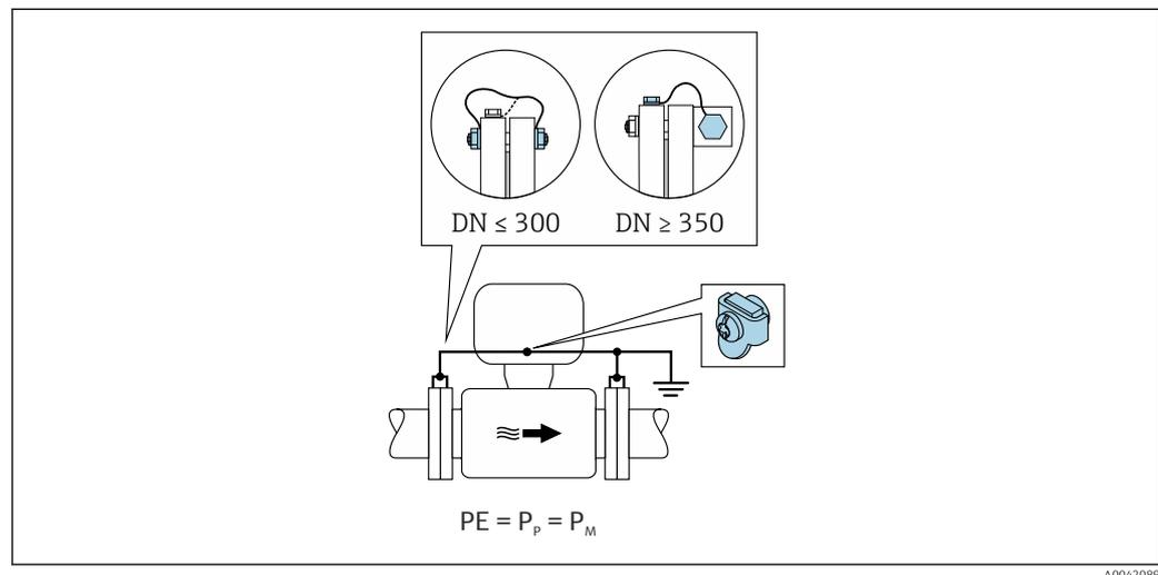
1. Connect both sensor flanges to the pipe flange via a ground cable and ground them.
