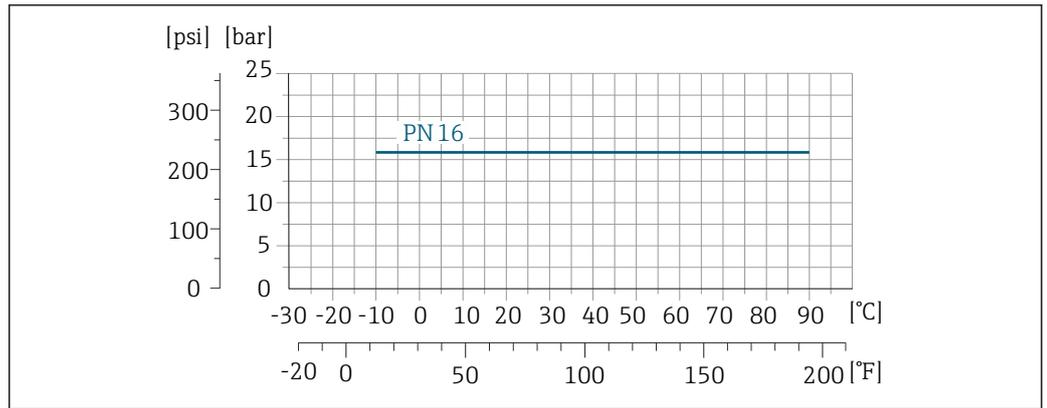
26 Process connection material: carbon steel
