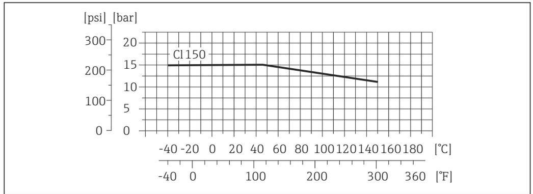
13 Process connection material: stainless steel, 1.4404 (F316L)
