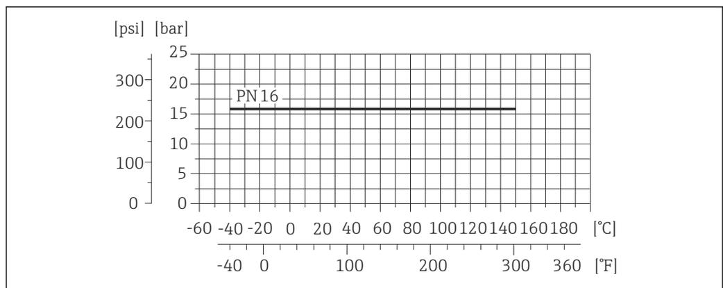
17 Process connection material: stainless steel, 1.4404 (F316L)
