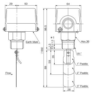
\*1 Connection screwed length to a Tee joint is 12 ±1.2mm.
