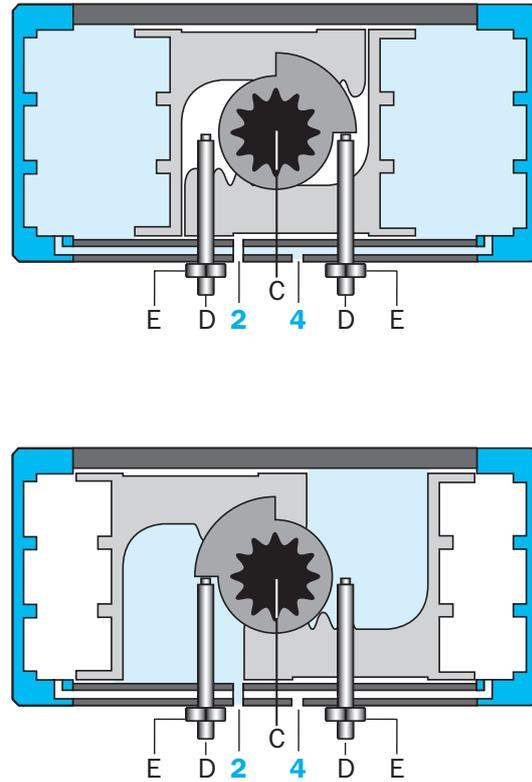
If the two outer chambers are pressurised via connection „4“, the pistons move towards each other into the basic position (0°). The force of both pistons is transmitted to the pinion „C“ via the racks. If connection „2“ is pressurised and connection „4“ is vented, the pistons move apart into the 90° position.
