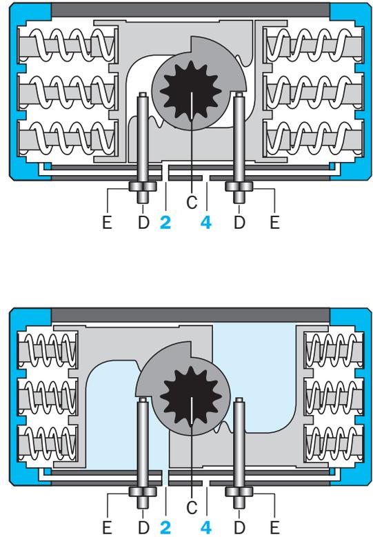
In the single-acting model the springs push the pistons back into the basic position and air is exhausted from connection „2“.
