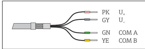
3 Sensor fixed cable with terminated cable cores
