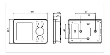
$N^{\circ}$  of settable temperatures = 3 Time slots = 0.5 hDifferential = 0,2 K Thermometer resolution =  $0,1^{\circ}C$ Thermometer precision =  $\pm 0.3$ °C Max. room temperature = 50°C Insulation class = II Protection rating = IP20 Options = 12h/24h clock and °C/°F selection Operating mode: Manual/Automatic/Anti-freeze System: heating/air conditioning Certifications = CE, ENECO3, EAC
