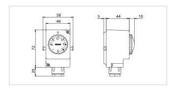
Differential =  $10\pm3$ K Max. head temperature =  $55^{\circ}$ C Protection rating = IP40 Electrical contact capacity = 10(2,5) A / 250 Vac Protection rating = IP40 Certifications = CE, ENECO3, EAC
