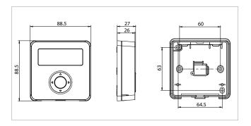
Regulation range =  $5^{\circ} \div 35^{\circ}C$  $N^{\circ}$  of settable temperatures = 2 Time slots = 1 hDifferential = 0,2 K Thermometer resolution =  $0.1^{\circ}$ C Thermometer precision =  $\pm 0.3$ °C Max. room temperature = 50°C Insulation class = II Protection rating = IP20 Options = 12h/24h clock and °C/°F selection Operating mode: Manual/Automatic/Anti-freeze System: heating/air conditioning Certifications = CE, ENECO3, EAC
