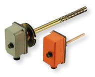
LSC1 is a boxed immersion thermostat, with liquid expansion probe, unipolar, safety temperature limiter with manual reset, fail-safe for capillary breakage, complete with watertight protection pocket. Useful in appliances where safety is required due to the temperature increase.
