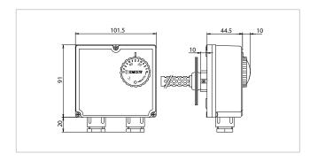
Electrical contact capacity = 10 (2,5) A / 250 Vac Adjustable temperature FAN = 0°/60°C Internal adjustable temperature LIM = 30°/120°C Protection rating = IP40 Max. head temperature = 80°C Max. bulb temperature = 150°C Certifications = CE, ENECO3, EAC
