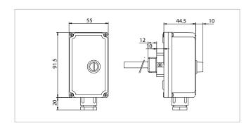
Electrical contact capacity = 10(2,5) A / 250 Vac Switches = interrupted due to temperature increase Thermal gradient = 1°K/min Max. head temperature = 80°C Max. bulb temperature = 125°C Protection rating = IP40 Certifications = CE, ENECO3, DIN, PED, EAC
