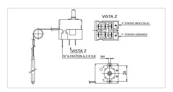
Electrical contact capacity = 15 (2,5) A / 250 Vac Switches = changeover Max. head temperature = 80°C Capillary length = 1500 mm PVC Min. capillary curvature radius = 5 mm Connection = via faston Certifications = CE, ENECO3, EAC
