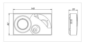
Electrical contact capacity = 5(1) A / 250 Vac Temperature range = 10° ÷30°C
