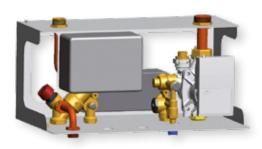
WATERWARM is a compact hydraulic kit, combined with a pellet stove or a thermo-fireplace, which allows the production of domestic hot water and water for heating. It includes a delivery/return group, a brazed exchanger with 20 plates, a diverter valve, a flow switch, an ErP circulator with degasser and built-in drain (only for code 561551) and a pre-wired electrical junction box. Includes white painted cover casing.
