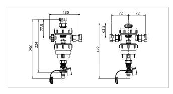
Max pressure = 3 bar Max. temperature =  $0 \div 90^{\circ}$ C Compatible fluids = Water and non-aggressive fluids Connections: G3/4" ISO228/1 female swivel captive nut hose fitting Ø15 mm Certifications = CE
