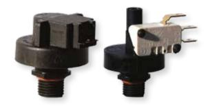
The pressure transducer consists of a Hall effect sensor that obtains an electrical signal proportional to the applied pressure. The pressure switch consists of a sensitive stainless steel element, for direct operation of a micro-switch for actuators or signalling devices. Transducers and pressure switches are generally installed in boilers and in appliances that need a pressure check.
