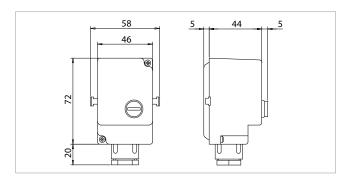
Temperature limiter pre-regulation =  $60^{\circ}$ C Regulation range =  $40^{\circ}$ ÷ $70^{\circ}$ C Tolerance = 0-10K Manual reset Reset temperature = -25K  $\pm$  8K range Max. head temperature =  $55^{\circ}$ C Electrical contact capacity = C-1: 0,5 A / 250 Vac C-2: 10(2,5) A / 250 Vac Protection rating = IP40 Certifications = CE, ENECO3, EAC
