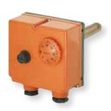
TLSC is a double boxed immersion thermostat, with liquid expansion probes, unipolar, temperature regulator and temperature limiter, fail-safe for capillary breakage, complete with watertight protection pocket. Particularly suitable for appliances where temperature control and safety is required.
