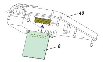
One module "Additional inputs / outputs"  ${\it 8}$  can be plugged onto main electronics  ${\it 40}$ :
