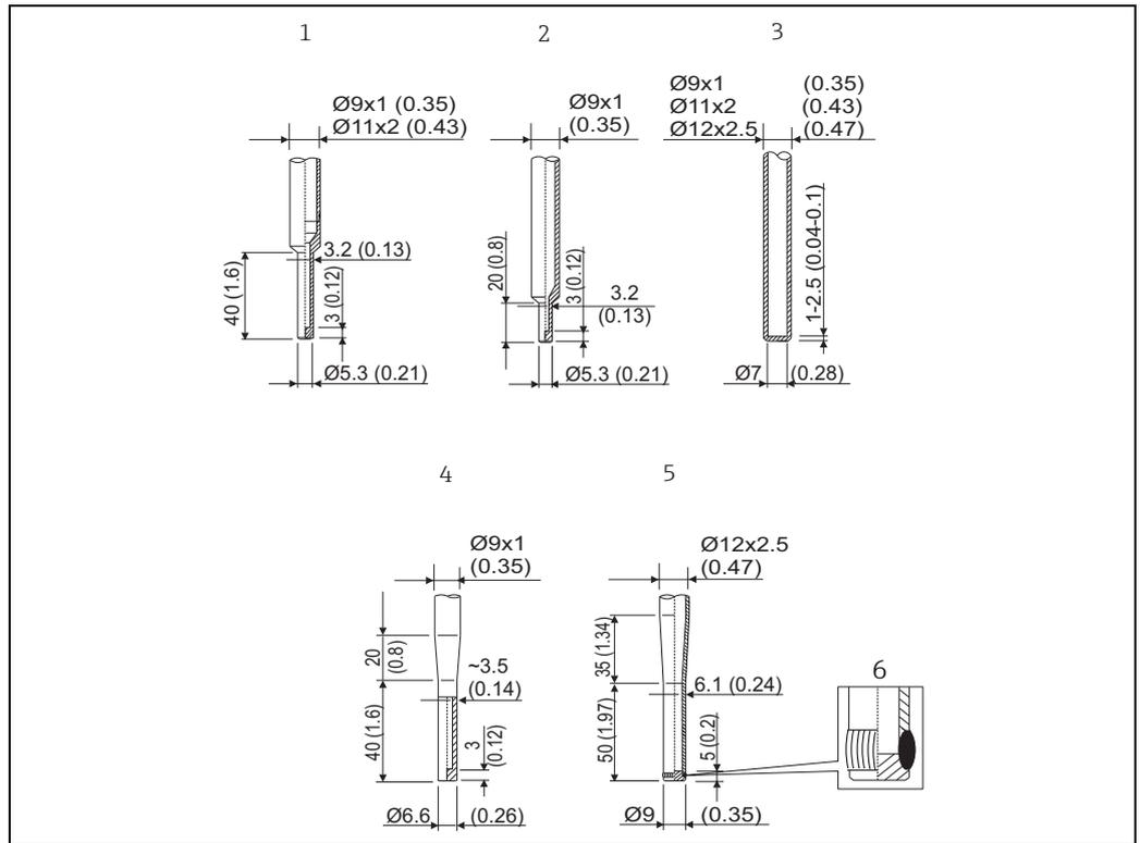
Available versions of thermowell tips (reduced, straight, tapered). Maximum surface roughness  $\leq Ra\ 0.8\ \mu m\ (31.5\ \mu in)$
