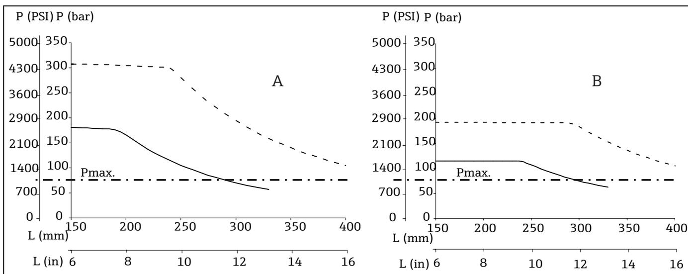
Maximum permitted process pressure for tube diameter, limited to 75 bar (1088 psi) by the threaded process connection
