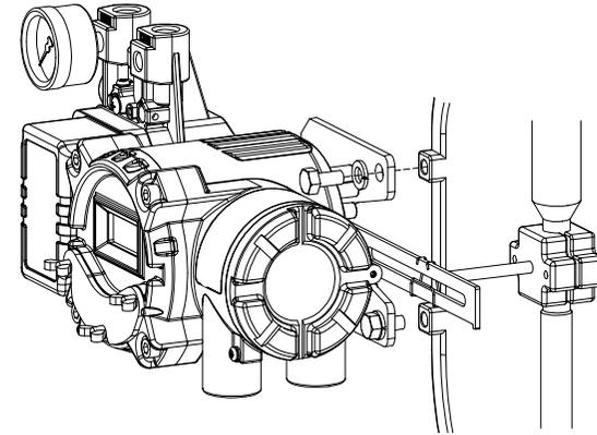
Installation of actuator clamp and connection bar
