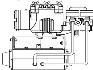
Piping connection example of YT-2400R with double acting actuator
