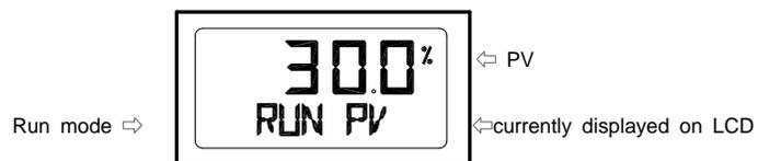
Run on the bottom line means that YT-2400 adjust valve stroke with receiving outside signal (4-20mA) and PV means the number on the LCD. In RUN mode, valve stroke is changed according to input signal. There are six types displayed in Run mode.
