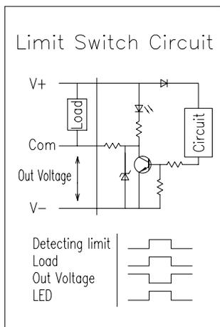
Terminal connection of limit switch
