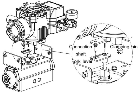
Fitting the pin on the YT-2400R main shaft into fork lever hole
