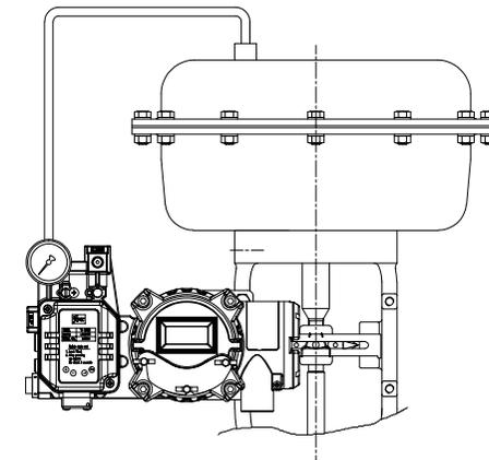
Piping connection example of YT-2400L with single acting actuator
