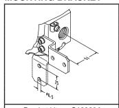
Bracket kit no. C139824 contains: Stainless steel 304 SS screws and bracket
