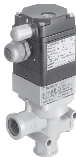
Fig. 2: 3/2-way solenoid valve · Actuated on one side · With spring return mechanism · K_{VS} 4.3 · G \frac{1}{2} connection
