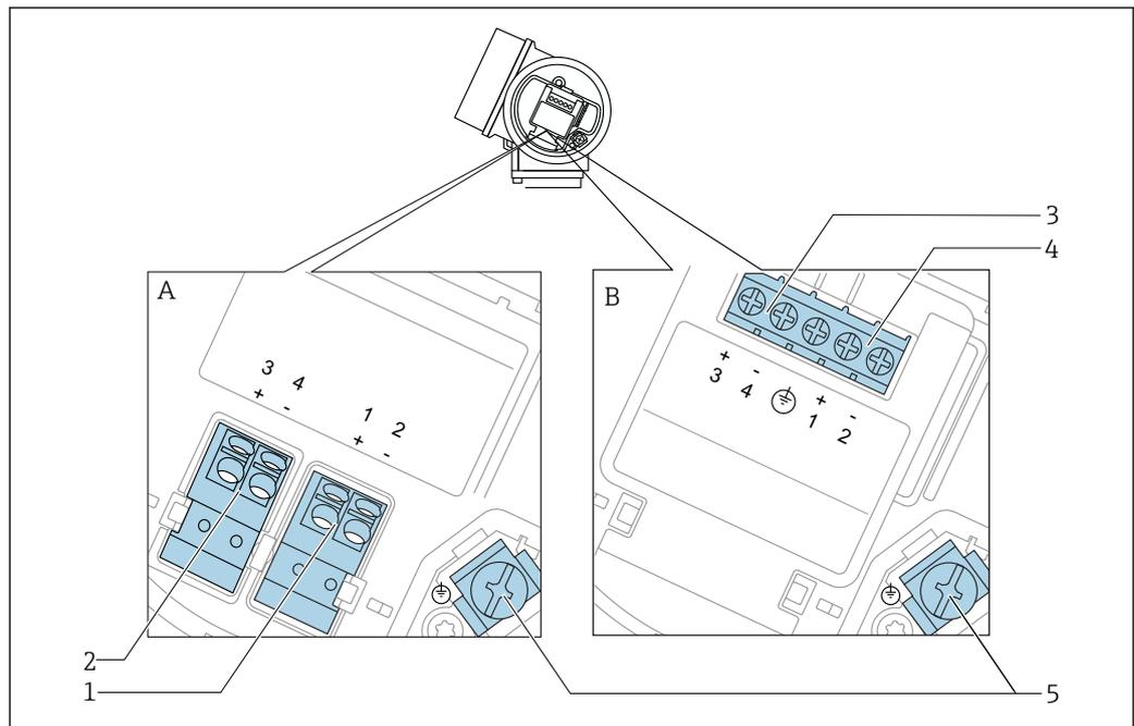
**14** Terminal assignment 2-wire: 4-20 mA HART, switch output
