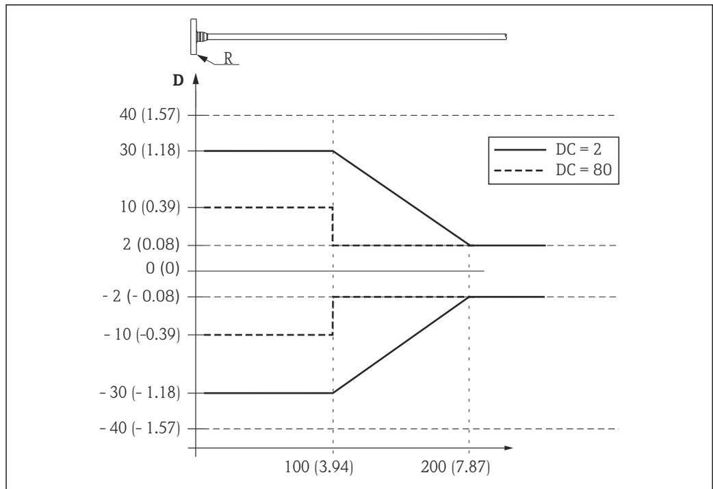
32 Measured error at the upper probe end; engineering unit: mm (in)
