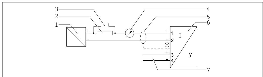
**15** Block diagram 2-wire: 4-20 mA HART, switch output
