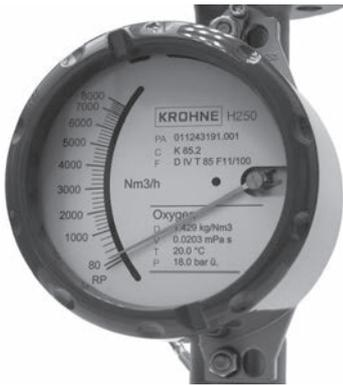
The usual measuring span of the H250 measuring device is 10 : 1.
