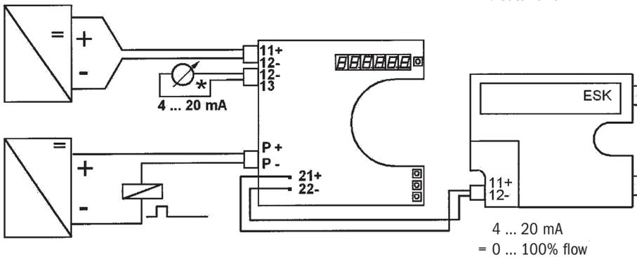
\* when metallically separated current evaluator modules (SPC) are used, the power supply (11/12) should not be grounded.
