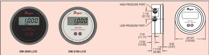
The Dwyer Series DM-2000 Differential Pressure Transmitter senses the pressure of air and compatible gases and sends a standard 420 mA output signal. The DM-2000 enclosure is specifically designed to mount in the same diameter cutout as a standard Magnehelic® gage. A wide range of models are available factory calibrated to specific ranges.
