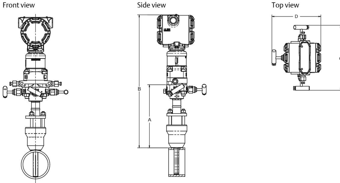
**Table 62: 3051CFA Annubar Flow Meter Dimensional Data**
