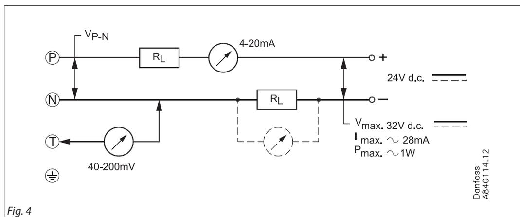
The transmitter has a wiring diagram, see fig. 4. Terminals P (positive) and N (negative) are connection terminals for the supply voltage. The same leads are used for supply voltage and output signal. A function test can be performed between terminals N and T without cutting off the current loop.
