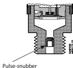
EMP 2 with the pressure range 0 – 6 bar and 0 – 10 bar at extended test pressure is provided with an integrated pulse snubber for protection of the sensor element against cavitations and air bubbles in the media due to extreme pressure peaks and pulsations. Such conditions may be caused by pumps or fast operation valves in both high and low pressure systems.
