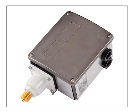
The RT-E series consist of pressure and differential pressure switches as well as thermostats. The units are designed for industrial refrigeration and general industrial application in explosive zones acc. to 2014/34/EU Atex directive, explosive zone 1, for surface equipment, category 2.
