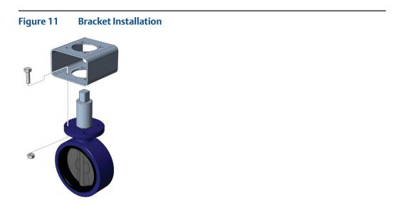
5. Install the actuator to the bracket. Tighten all bolts and apply the correct torque (refer to Table 8).
