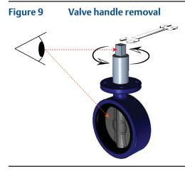
When required, check if the insert drive (23) is mounted. If not, use a plastic mallet and tap slightly until the reducer square is in the required position.
