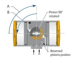
A = Rotation when central air chamber is pressurized.
