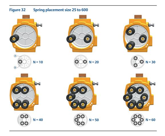
A = Piston top view B = Position of gear rack
