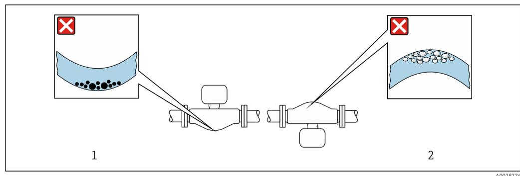
☑ 22 Orientation of sensor with curved measuring tube
