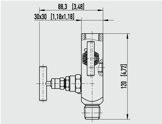
Plug screw for venting connection is included in delivery, though not pre-fitted.
