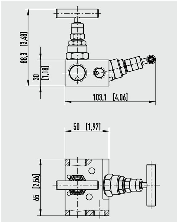
Plug screw for vent connection is included in delivery, though not pre-fitted.
