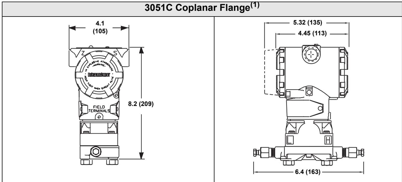
(1) For FOUNDATION fieldbus and Profibus PA transmitters with LCD Display, housing length is 5.78 in. (147 mm).
