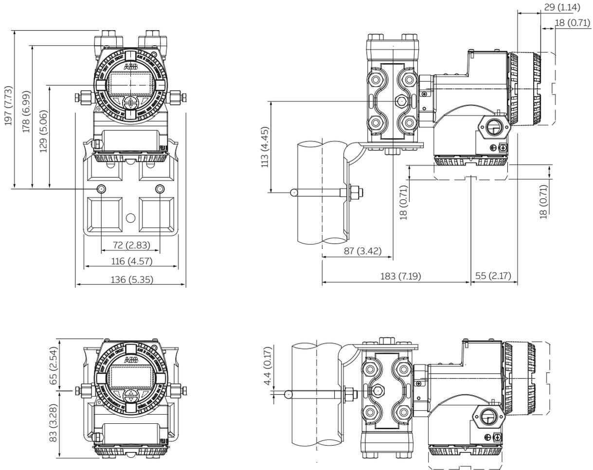
Figure 6 Transmitter with DIN aluminium housing - horizontal flanges on bracket for vertical or horizontal 60 mm. (2 in.) pipe mounting
