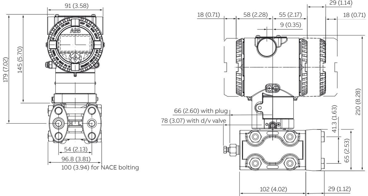
Figure 2 High static transmitter with barrel housing - horizontal flanges
