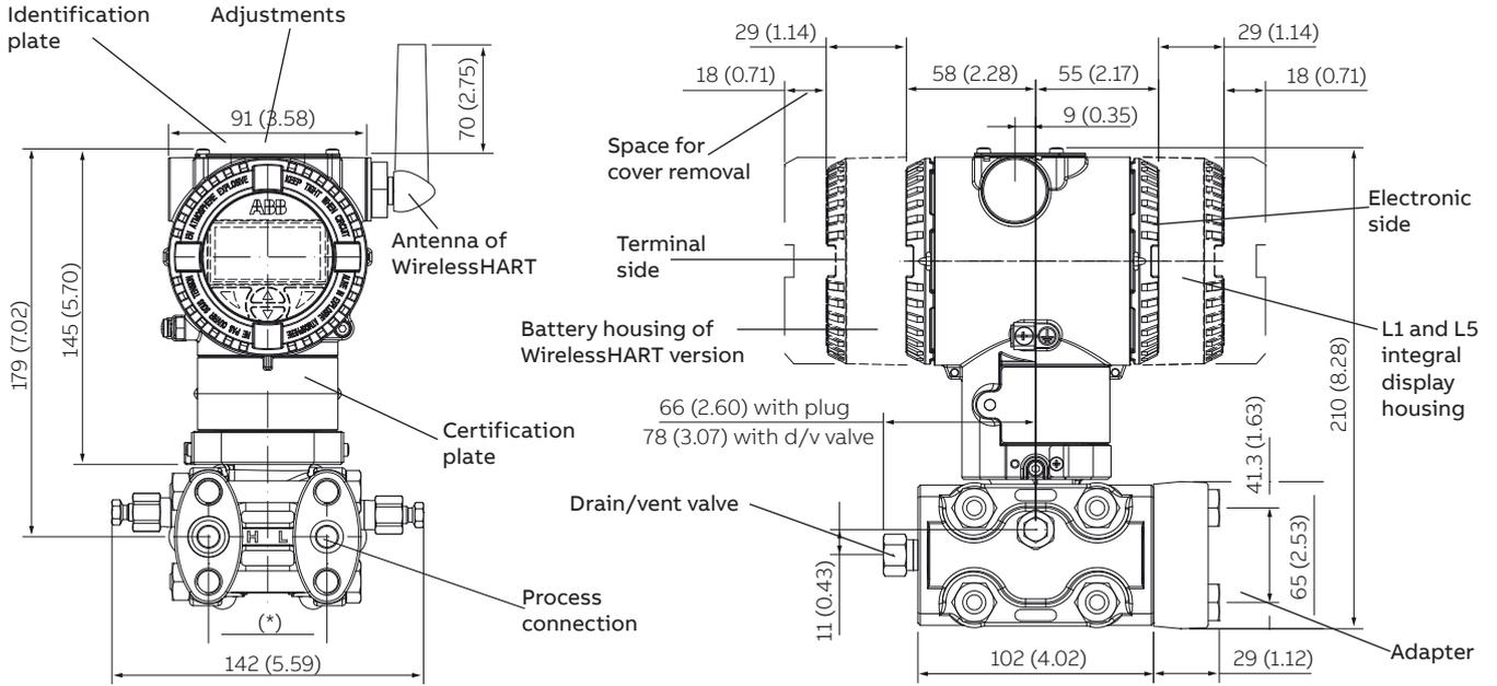
(\*) 54 (2.13) mm (in) on 1/4 – 18 NPT process flange; 51 (2.01), 54 (2.13) or 57 (2.24) mm (in) according to 1/2 – 14 NPT adapters fitting 54 (2.13) mm (in) with negative side provided with a removable filter for gauge measurement (version 266DSHxP)
