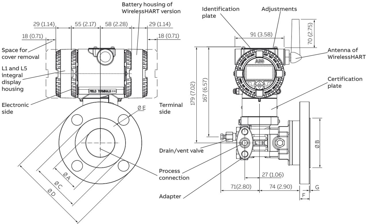
Figure 9 Transmitter with barrel housing - flange mounted version
