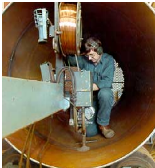
شکل ۱-۵ submerged arc welding (SAW)
